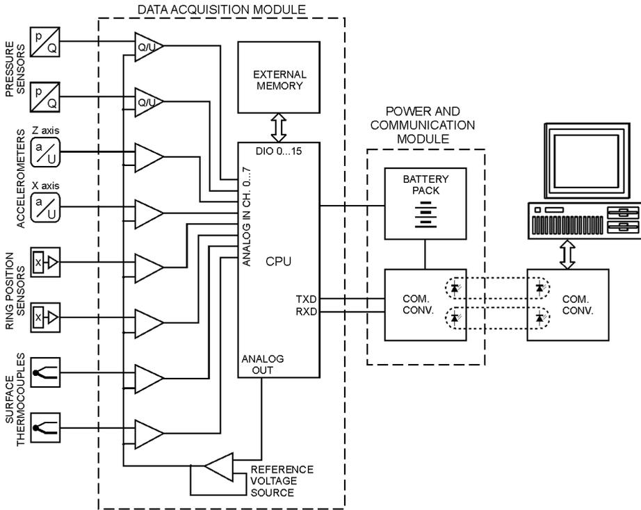
Fig. 2. Block diagram of movable data acquisition system
