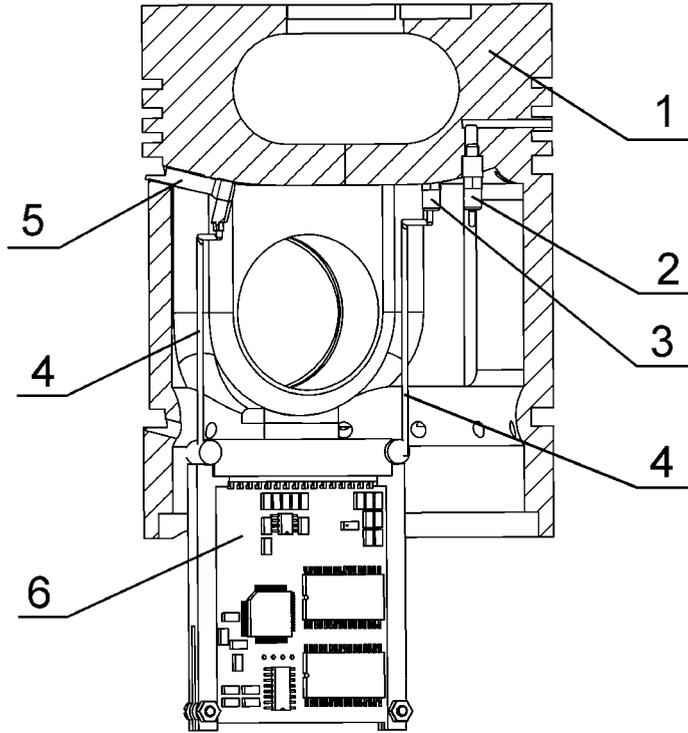
Fig. 3. Arrangement of electronic devices in the research piston
