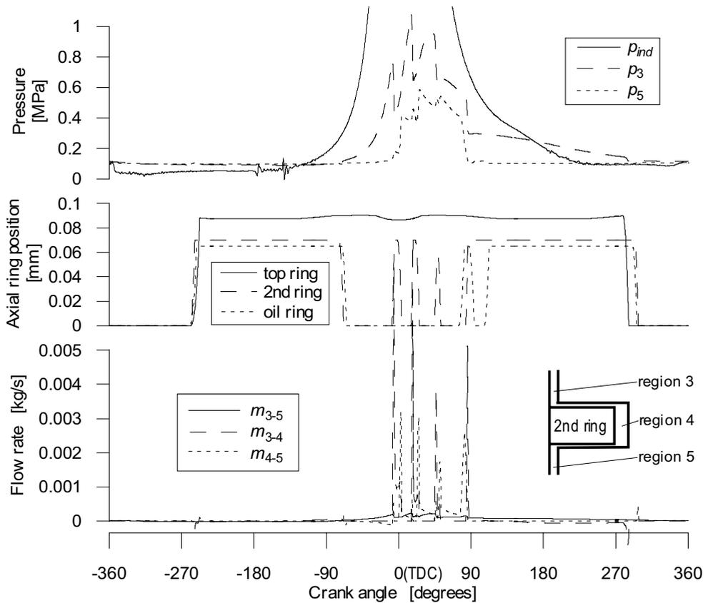
Fig. 1. Pressures ( $p_{ind}$  – in the combustion chamber,  $p_3$  – in the land between the top and the second ring and  $p_5$  – in the land between the second and the oil ring), axial positions of rings in their grooves (value zero means, that ring adheres to upper groove flank) and intensities of gas flow through crevices of second compression ring ( $m_{3-5}$  – through the ring-end gap,  $m_{3-4}$  and  $m_{4-5}$  through crevices between the ring and the groove)
